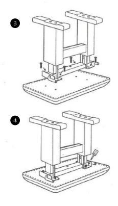
Bolt bench frame to bottom of bench top as shown
